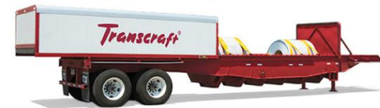
Transcraft offers specialty solutions to meet unique application requirements. Our coil haulers provide the lowest available center of gravity for reliable hauling and handling of steel coils.
